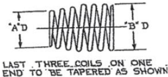
The first thing to note is that the spring rate changes at the two lengths. At the first length (0.5"), we have a rate of  $3/(0.696 - 0.5) = 15.306$  lbf/in. Then using the two length/load requirements, we have a rate of  $(5-3)/(0.5-0.375) = 16$  lbf/in. This means that the coil(s) with the largest OD must have deflected to solid before the second load point because the rate will remain constant until that occurs.
